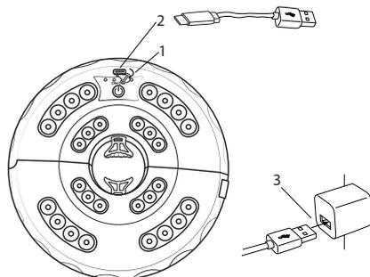
*Note: All 4 indicator LEDs will remain lit when the battery is fully charged.*
