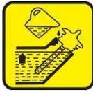
The oil filler opening is located here. Fill up to level indicated.
