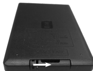
Figure 9: Unlocking the battery holder
