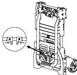
⑨ Push the handle slightly forward and backward when press the levers to unlock and fold handle down.
