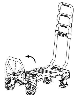
④ Press levers to unlock handle and raise to desired height. Lift the base plate if more load control is desired.
