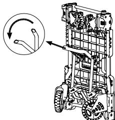
① Pull handle down to lock wheels in place.
