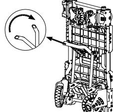
⑩ Press levers and lock handle in folded position.
