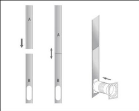
4. Close your window to secure the kit in place. It needs to hold the windows kit firmly in place, secure the window kit with duct tape if required. It is recommended that the gap between the adapter and the sides of the window should be sealed off for maximum efficiency.
