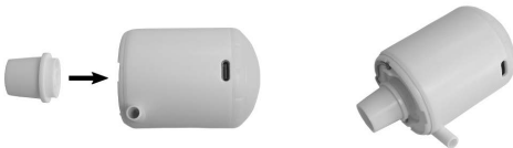
Fig. 4: Attaching the adapter to the intake opening
