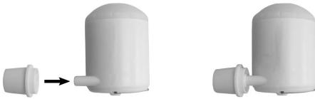
Fig. 2: Attach adapter to pump outlet
