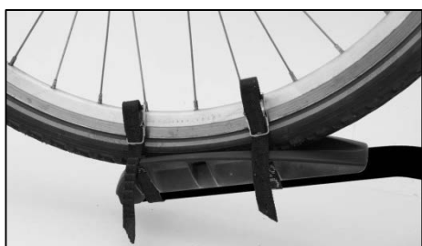
Figure 16: Tensioning straps for front wheel
