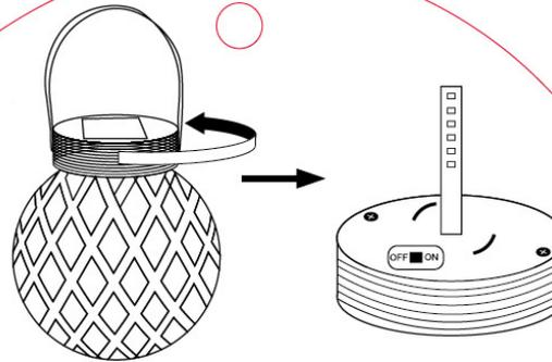
1. There is an 'ON/OFF' switch at the bottom, press it to 'ON' position.
